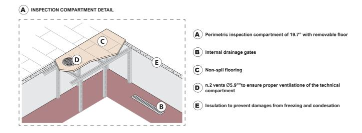
NB: we recommend to let the spa discharge its weight on the base and not on the edges. We advice to fix the last line of tiles near the edge once the installation is finished, the result will be a good match between the spa and the covering.
