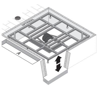
Optional lift with removable inspection hatch "A" positioned on the side where the components of the spaare situated.
